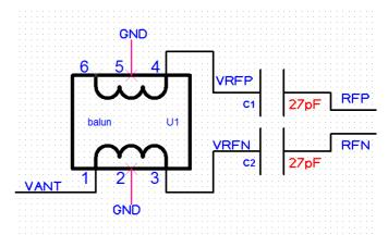
Note that in this configuration pin 2 of the balun is grounded, while pin 6 is not connected.
