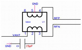
Note that in this configuration pin 2 of the balun is connected to a RF capacitor that maintains the correct common-mode bias point, while pin 6 is not connected.
