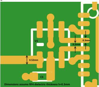
The dimensions given in the layout above assume that the RF ground layer is a solid sheet of metal 0.3mm below the top layer shown.
