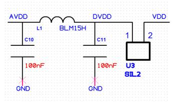
Note that the ground used for C10 (AVDD) should refer to the Analog ground domain, while the ground used for C11 (DVDD) should should refer to the Digital ground domain.
