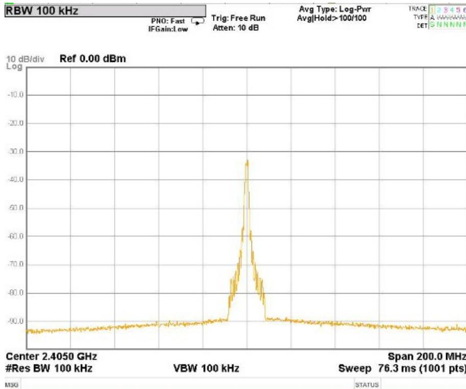
Figure 7.1: EXG Wideband PSD,  $F_c \pm 100$  MHz
